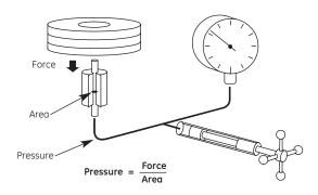
The pressure is measured when placed on a correctly spinning and floating piston. The total pressure measured is the summation of the weights plus the piston weight carrier assembly.
